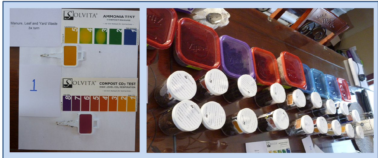
Fig. 9. Comparing the indicators to the colour charts when using the Solvita test kits at home
