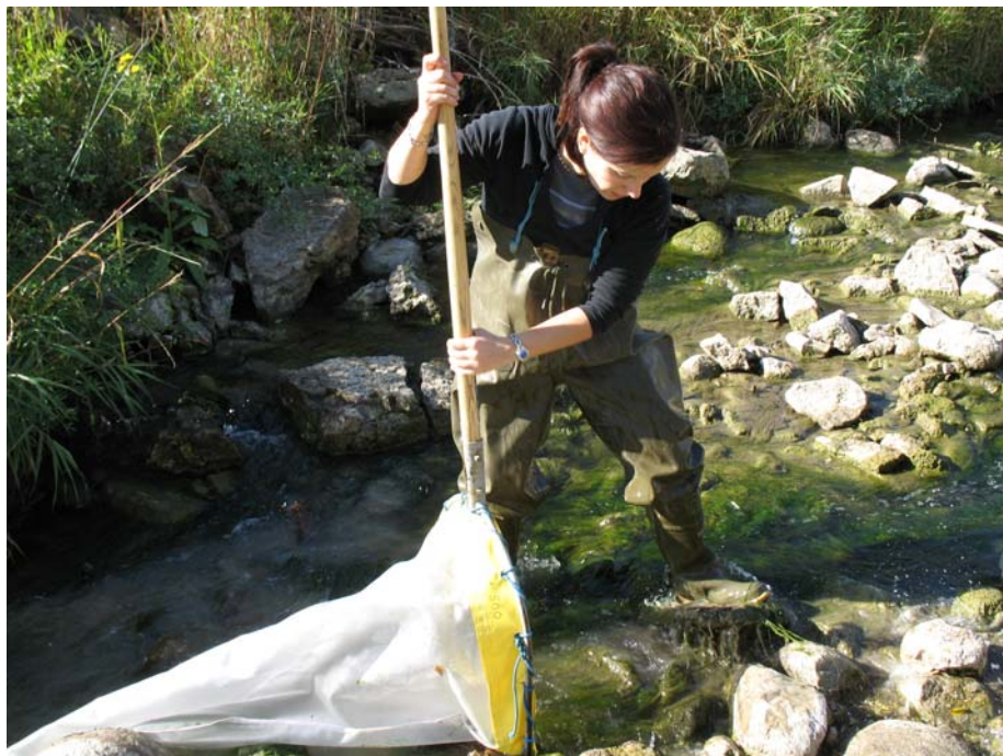
Photo 4. Example of kick net used and collection of invertebrates by technician.
