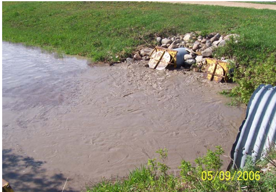
Photo 14. Shurkas Drain and roadside ditch where a turbidity reading was greater than 1000 NTU.
